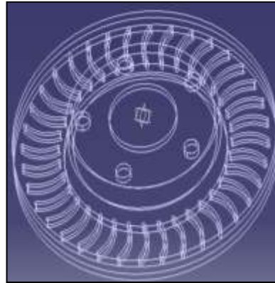
Fig.5 Rotor with Forward Curved Fins
