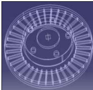
Fig.3 Rotor with Straight Elliptical Fins
