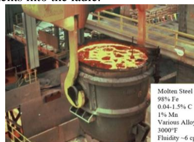
Figure 1. ladle containing molten steel, adapted from [2].
