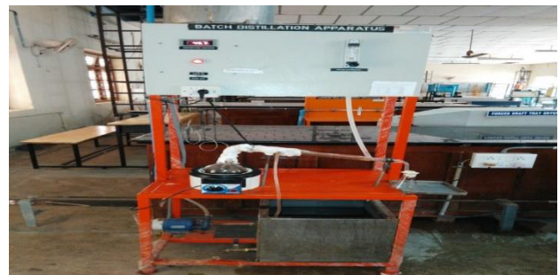
Figure 2. Batch distillation apparatus
