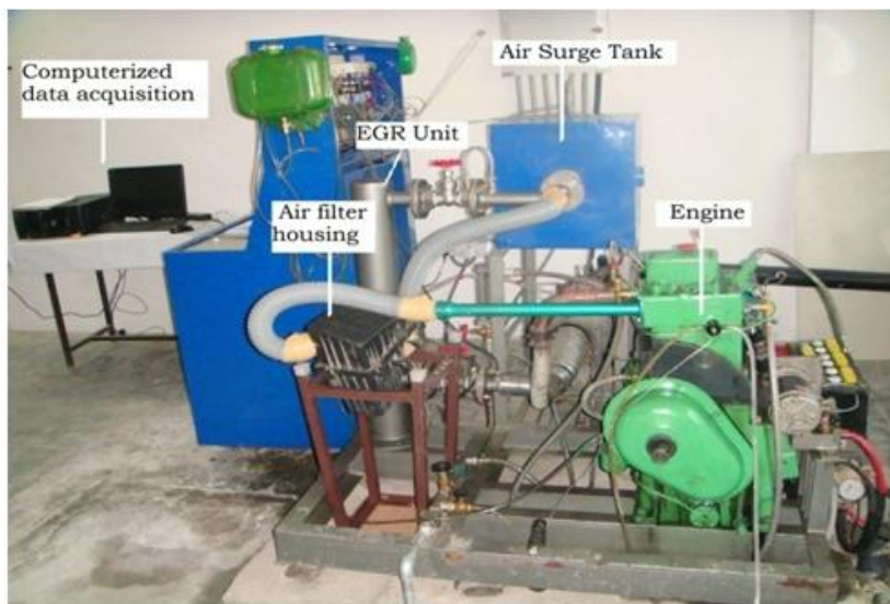
Fig: 2.2 Photographic View of Computerized Diesel Engine Setup with Air Filter Housing Arrangements and EGR Facility
