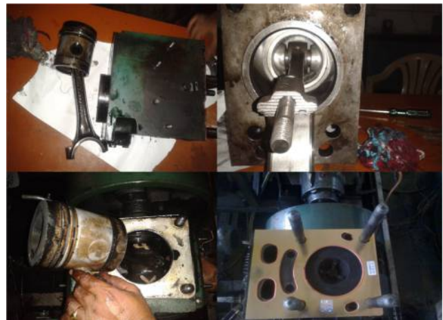
Figure 4 Modified piston arrangement in-cylinder
