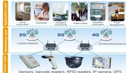
Figure 3. IOT architecture with example devices in each layer [10]
