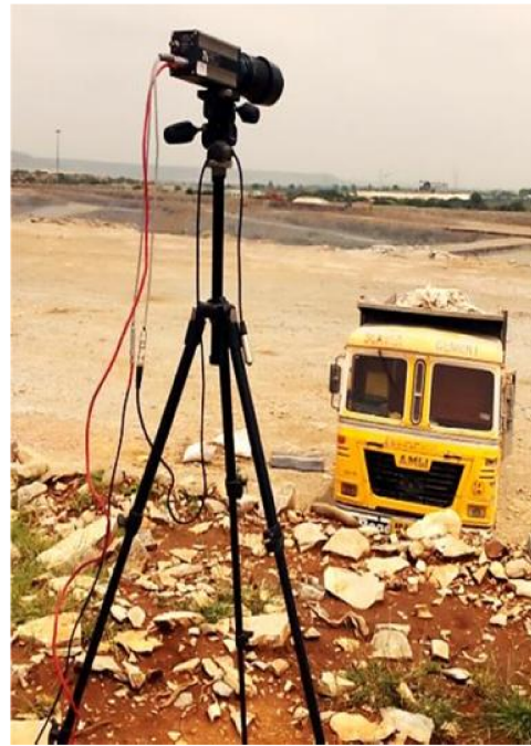
Figure 2: High speed video camera of 1000fps capacity
