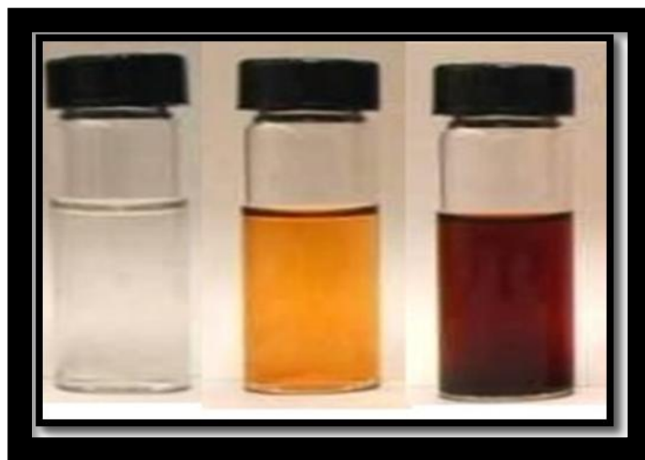
Fig. 2 Synthesis of silver nanoparticles using Gymnosporia emarginata young leaves extract treating with AgNO 3 solution at room temperature
