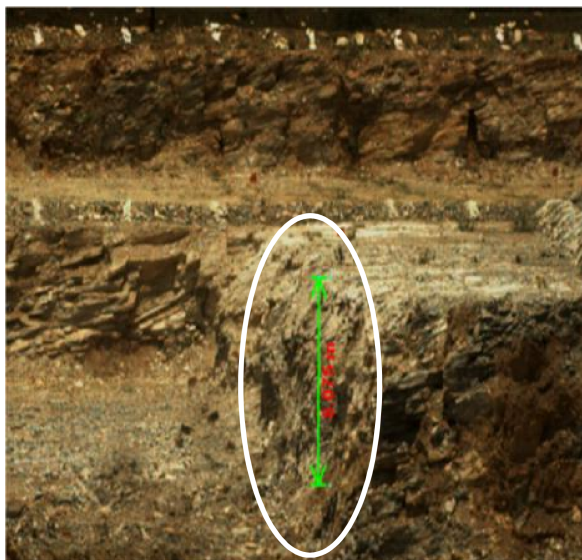
Height of the bench obtained as 8.075m
